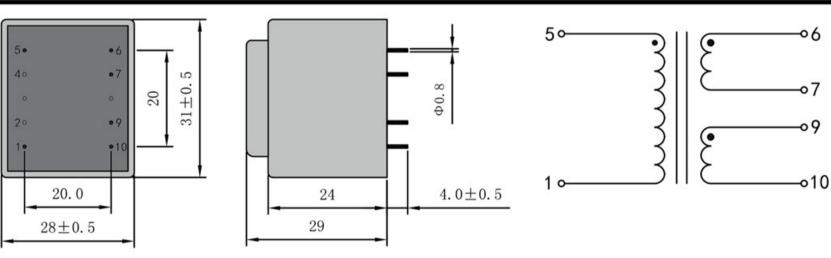
Dimensions with no indication of tolerances: ± 0.3mm Custom-made transformer also will be welcome.
