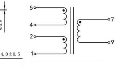
Dimensions with no indication of tolerances: ± 0.3mm Custom-made transformer also will be welcome.
