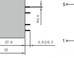
Dimensions with no indication of tolerances: ± 0.3mm Custom-made transformer also will be welcome.
