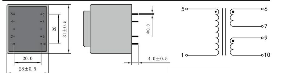
Dimensions with no indication of tolerances: ± 0.3mm Custom-made transformer also will be welcome.
