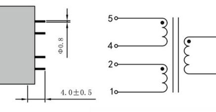
Dimensions with no indication of tolerances: ± 0.3mm Custom-made transformer also will be welcome.
