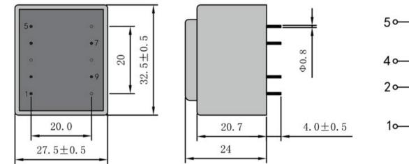
Dimensions with no indication of tolerances: ± 0.3mm Custom-made transformer also will be welcome.
