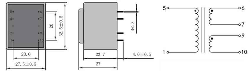
Dimensions with no indication of tolerances: ± 0.3mm Custom-made transformer also will be welcome.
