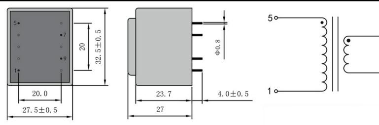
Dimensions with no indication of tolerances: ± 0.3mm Custom-made transformer also will be welcome.
