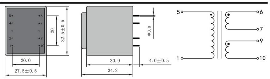
Dimensions with no indication of tolerances:  $\pm$  0.3mm Custom-made transformer also will be welcome.
