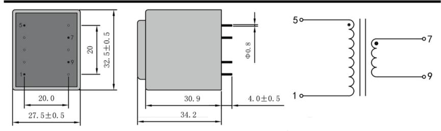
Dimensions with no indication of tolerances:  $\pm$  0.3mm Custom-made transformer also will be welcome.
