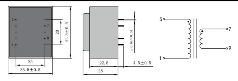
Dimensions with no indication of tolerances: ± 0.3mm Custom-made transformer also will be welcome.
