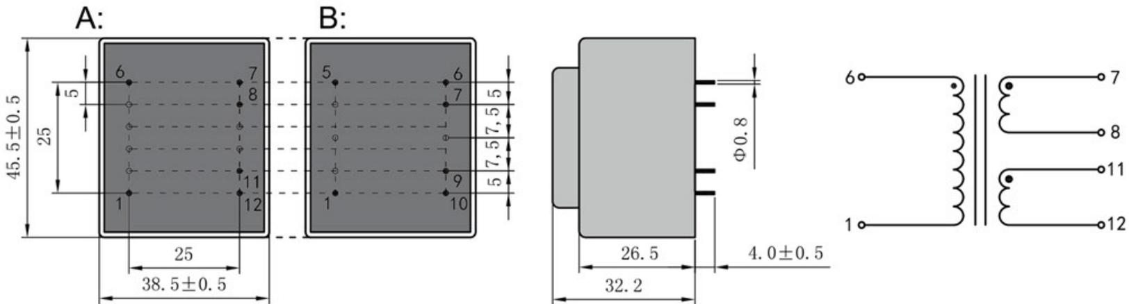
Dimensions with no indication of tolerances: ± 0.3mm
