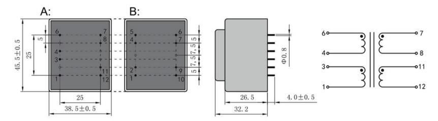
Dimensions with no indication of tolerances: ± 0.3mm Custom-made transformer also will be welcome.
