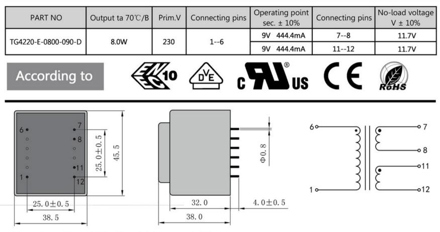
Dimensions with no indication of tolerances:  $\pm$  0.3mm Custom-made transformer also will be welcome.
