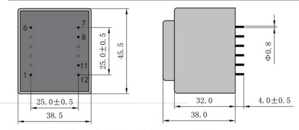
Dimensions with no indication of tolerances: ± 0.3mm Custom-made transformer also will be welcome.
