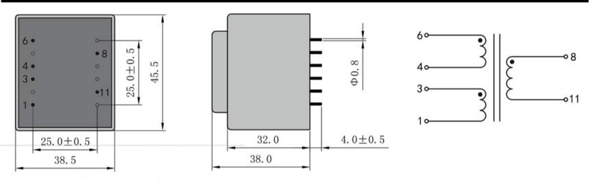
Dimensions with no indication of tolerances: ± 0.3mm Custom-made transformer also will be welcome.
