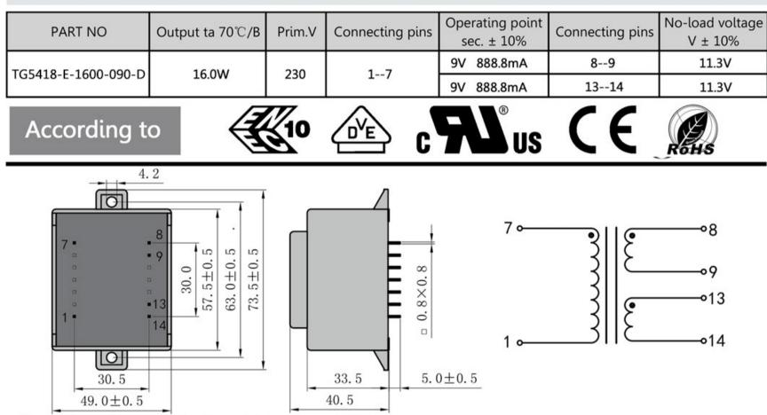
Dimensions with no indication of tolerances:  $\pm$  0.3mm Custom-made transformer also will be welcome.
