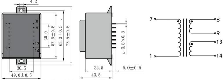
Dimensions with no indication of tolerances: ± 0.3mm Custom-made transformer also will be welcome.
