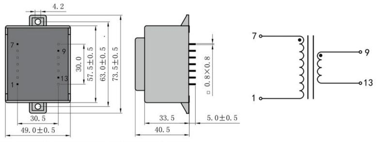
Dimensions with no indication of tolerances: ± 0.3mm Custom-made transformer also will be welcome.
