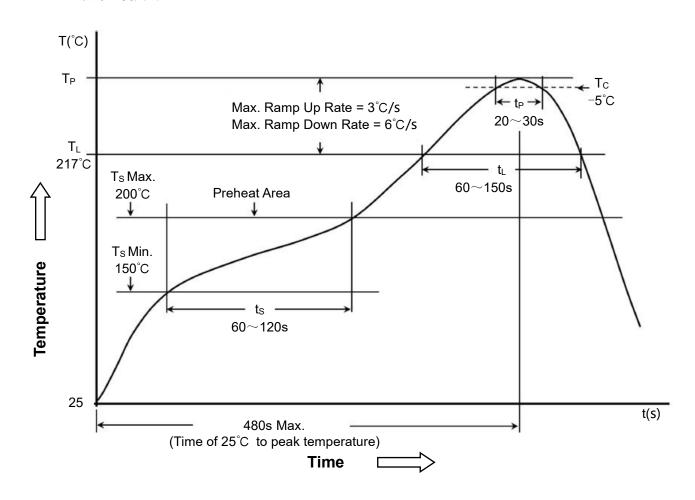
8.2 Classification of peak package body temperature  $(T_P)$  封装体峰值温度 $(T_P)$ 分类
